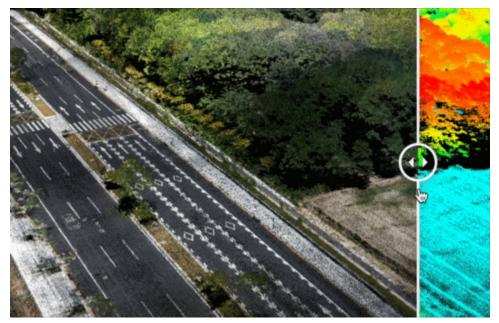
Nano P60 combines lidar point clouds with RGB imagery to generate high-density, high-precision 3D imaging with color by elevation features. Image courtesy of LidarSwiss.
